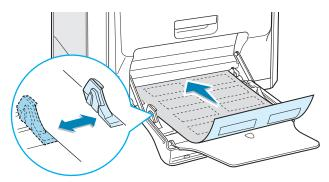
**3** When you print, configure the paper source to **MP Tray**, the paper type to Labels and the size in the software application. For details, see page 4.7.
